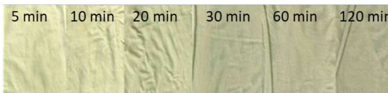
Fig.2 Cotton textile samples dyed with Yerba Mate extract (EM1): effect of dyeing time
