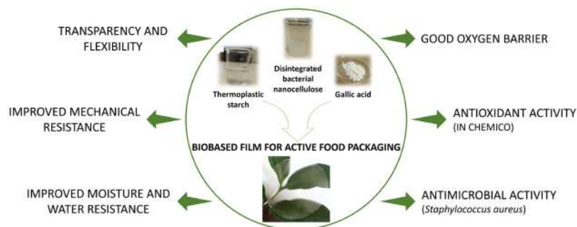
Figure 2- Scheme summarizing the fabrication of TPS_BNS_gallic acid-based films (Almeida, 2023).
