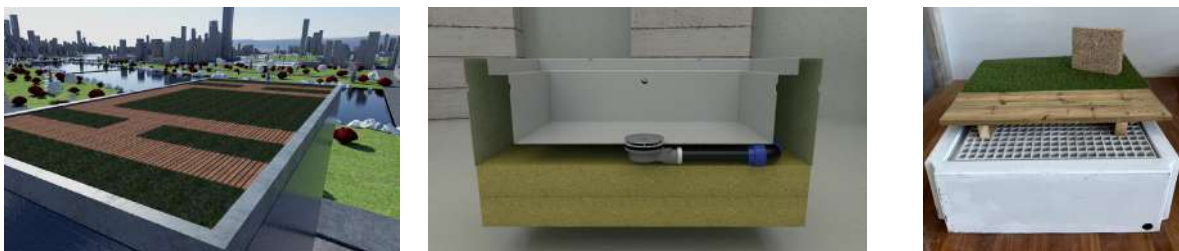
Fig. 2 ADAPTIVE: Retrofit of a building roofing with a gardened leisure space using the lightweight composite
