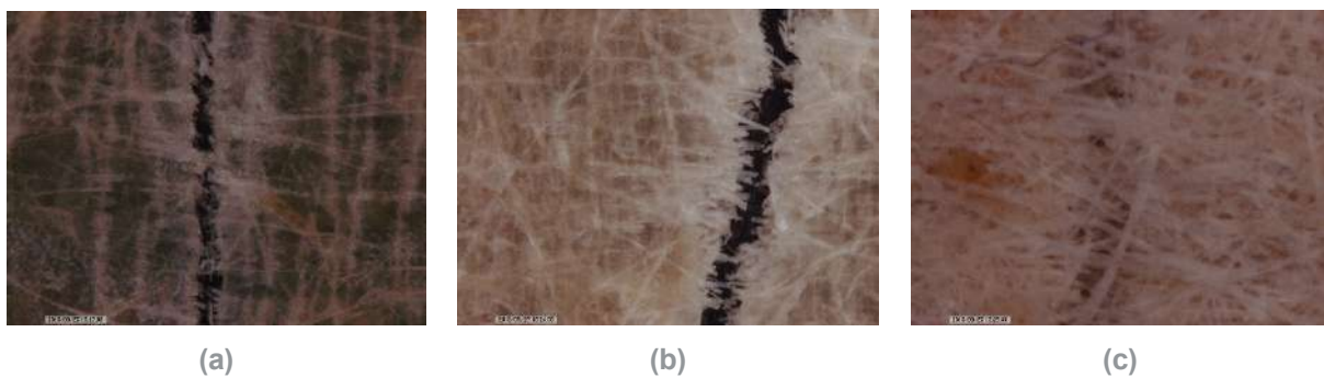
Microscopic images of tensile failure of biocomposites prepared with 10 % (a), 50 % (b), and 90 % (c) nettle fibers by weight
