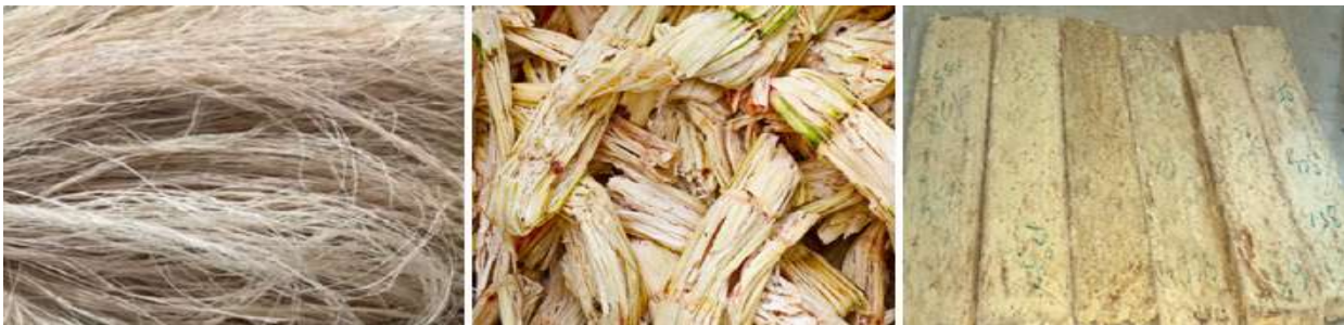
Figure 1: (a) Banana fibre (b) sugar cane bagasse fibre (c) Composite sheet
