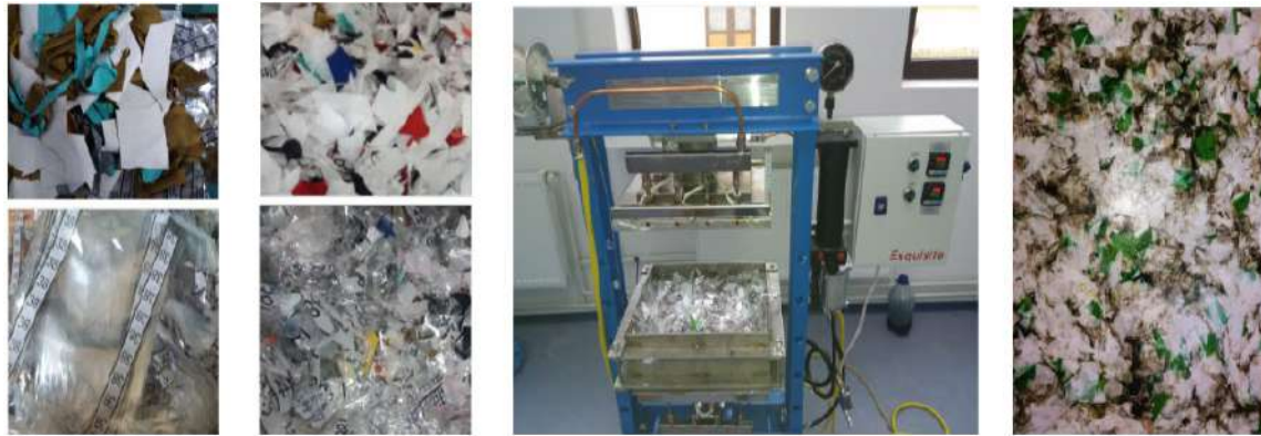
Fig.1 Technological process for producing waste-based composite material
