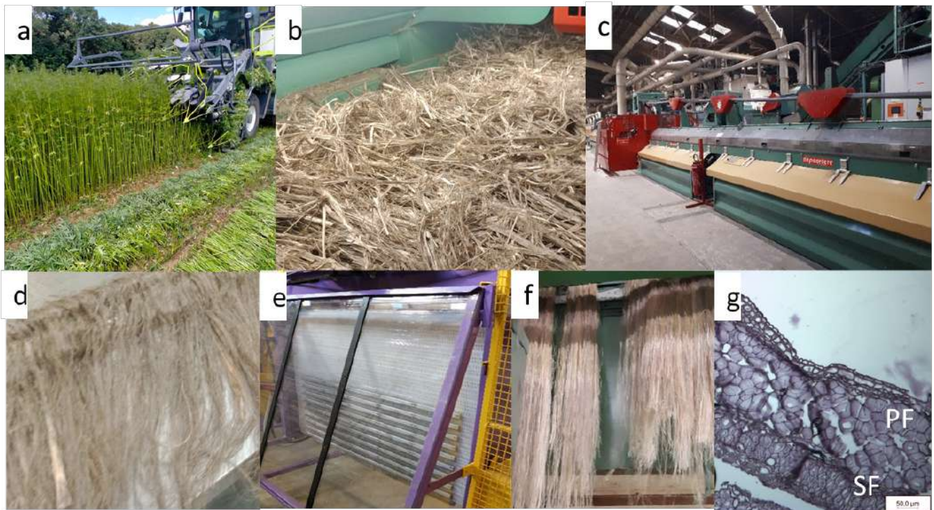
Fig.1: (a): Industrial hemp dedicated harvesting machine, (b) Hemp dew retted straw at the scutching input, (c) Industrial scutching machine, (d) Scutched long hemp fibres, (e) Labscale hackling machine, (f) Hackled hemp fibres, (g) histological cross section of a hemp stem
