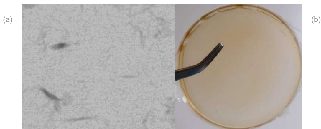
Fig.1 a) STEM micrograph of the extracted CNCs (50 000×). Scale bars represent 2 μm.
